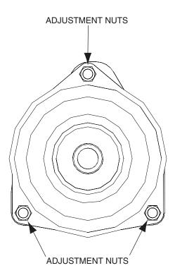
Figure 6-12. Clutch Air Gap Adjustment
